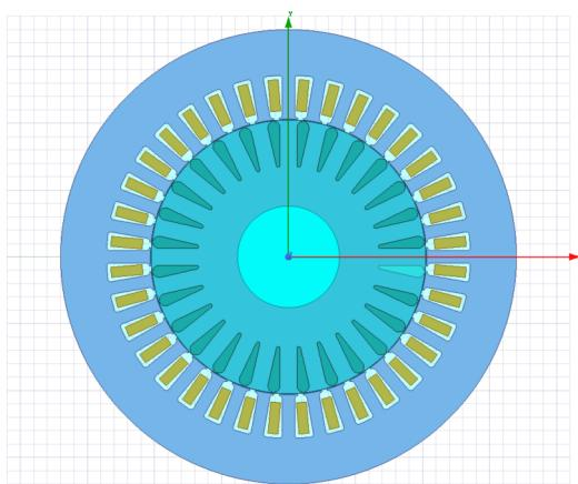
(a) 2D model elektromotora
