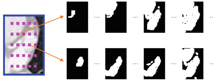
Figure 3.50: Generated segmentation proposals. The small magenta squares in the leftmost image represent different foreground seed points (seed hypothesis) for the graph-cut method. The bold blue lines surrounding the image represent the negative (background) seeds. For every seed hypothesis, the method creates a set of segmentation proposals with different \lambda values ( \lambda increases from left to right). The image shows two generated proposal sets for two seed hypotheses (orange arrows). Image source: Wang et al. [177].
