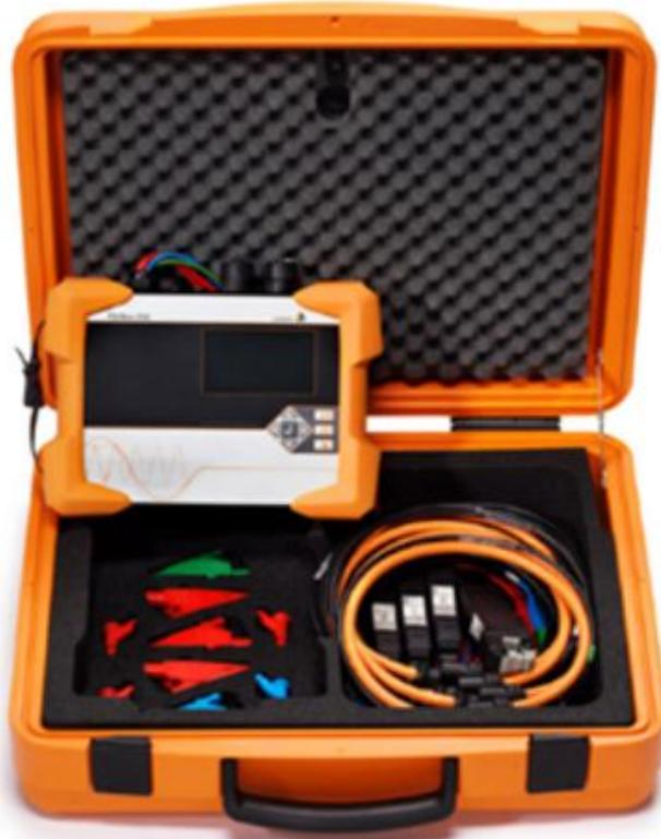
Slika 4.1. Mjerni instrument a-eberle PQ – Box 200 [13]
