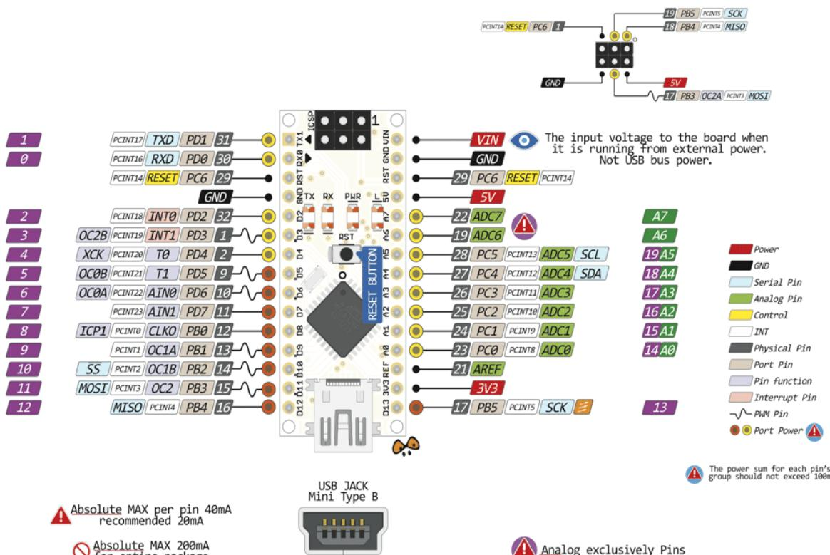
Slika 2.1. Arduino Nano raspored pinova.<sup>2</sup>
