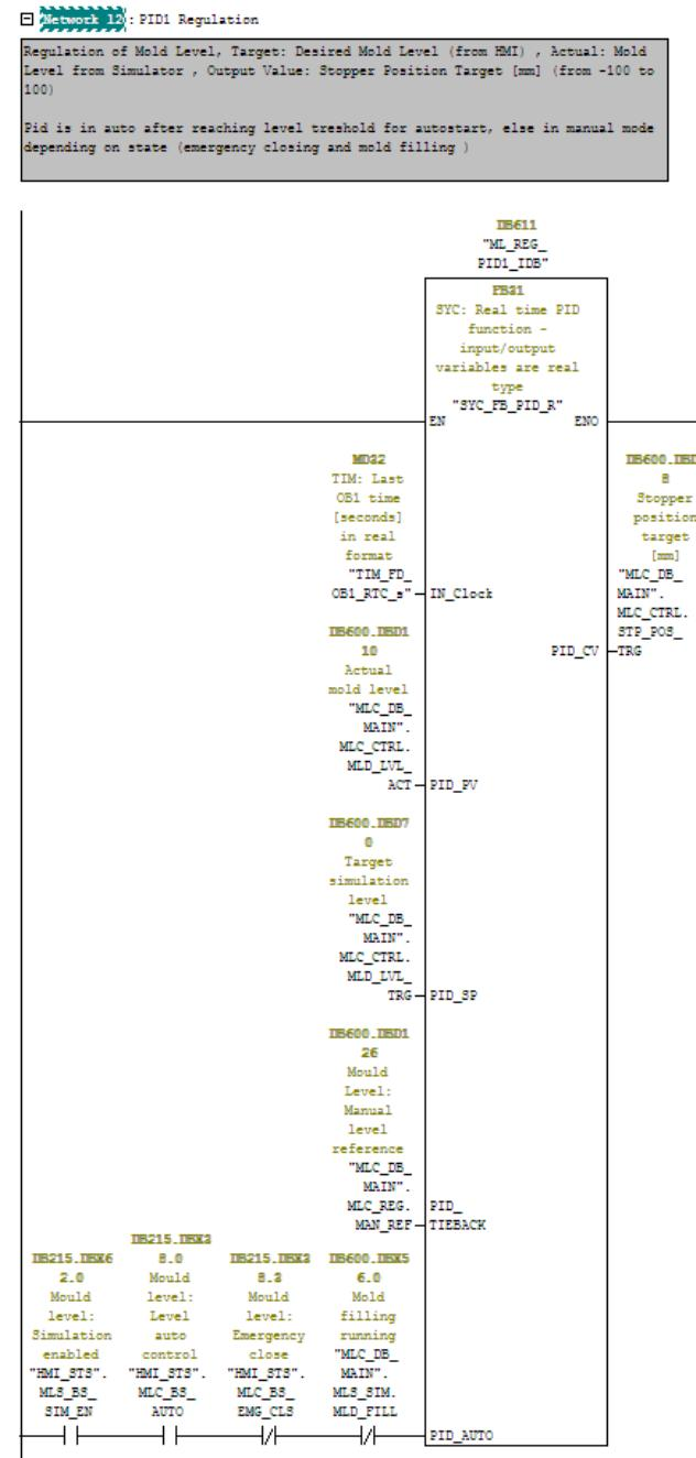
**Sl. 3.10. PID regulator razine čelika u kalupu.**
