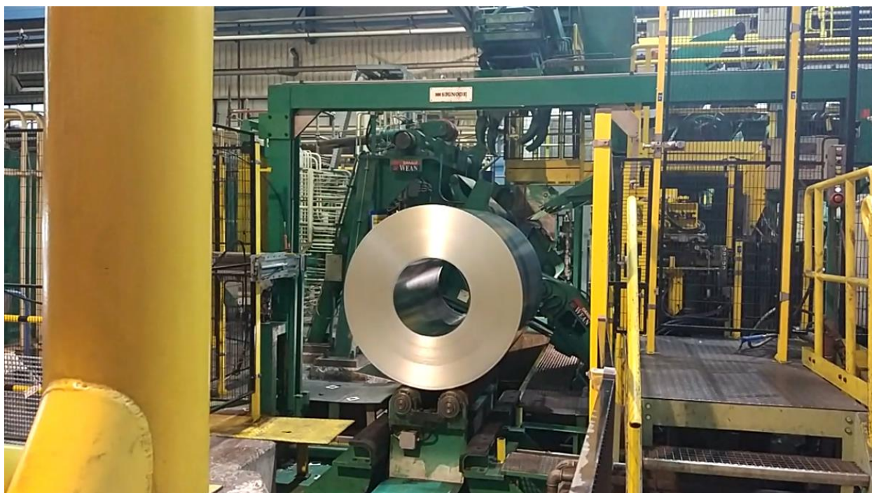
Sl. 3.2. Transport kotura
