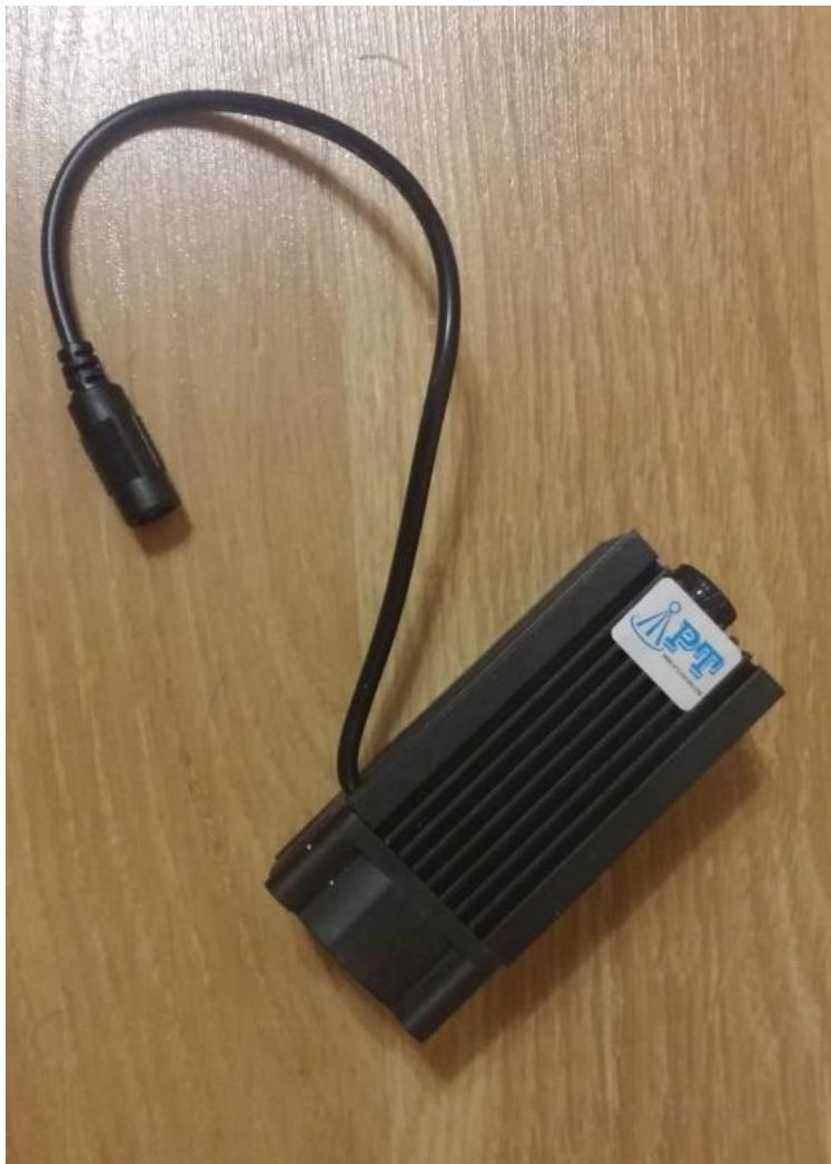
*Slika 3.10: Laser 2500 mW, 445 nm*
