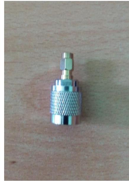
Slika 2.9. Adapter SMA<sub>m</sub>/N<sub>f</sub>
