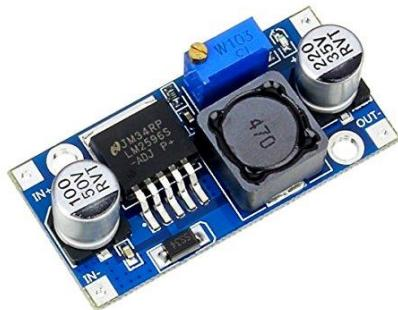
**Slika 4.6. LM2596 DC to DC *buck converter***
