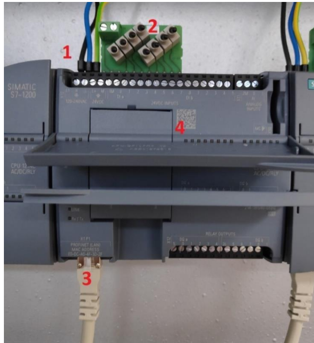
Slika 2.9 S7 – 1200 CPU 1214C AC/DC/Relay
