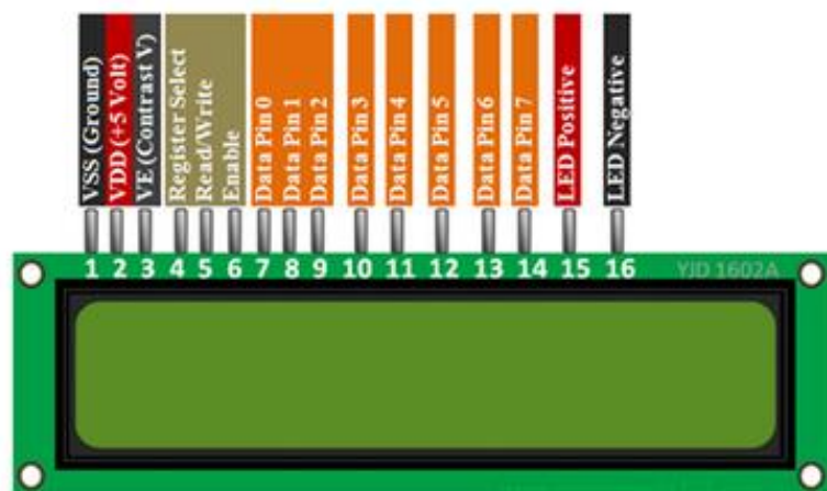
Sl. 3.16. Raspored pinova na LCD ekranu 19
