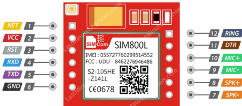
Sl. 3.8. Raspored pinova na SIM800L modulu 11
