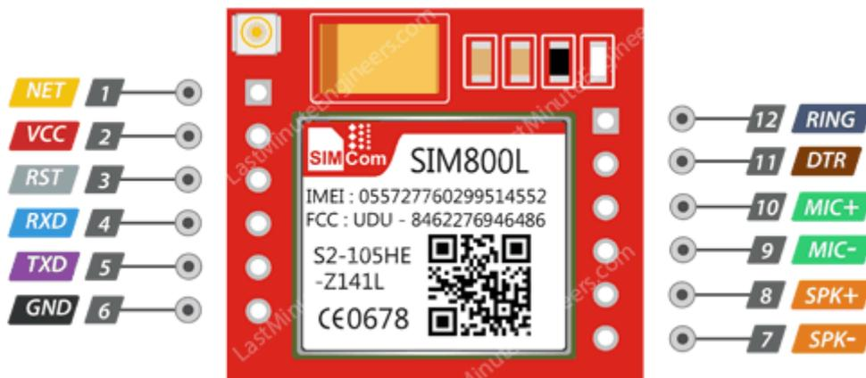
Sl. 3.8. Raspored pinova na SIM800L modulu<sup>11</sup>
