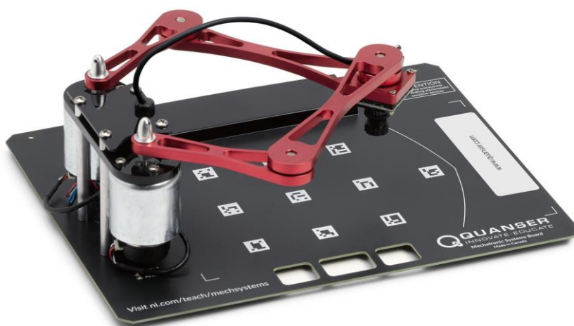
Slika 4.3. Quanser Mechatronics Systems Board [19]
