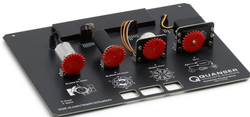
Slika 4.2. Quanser Mechatronics Actuators Board [18]
