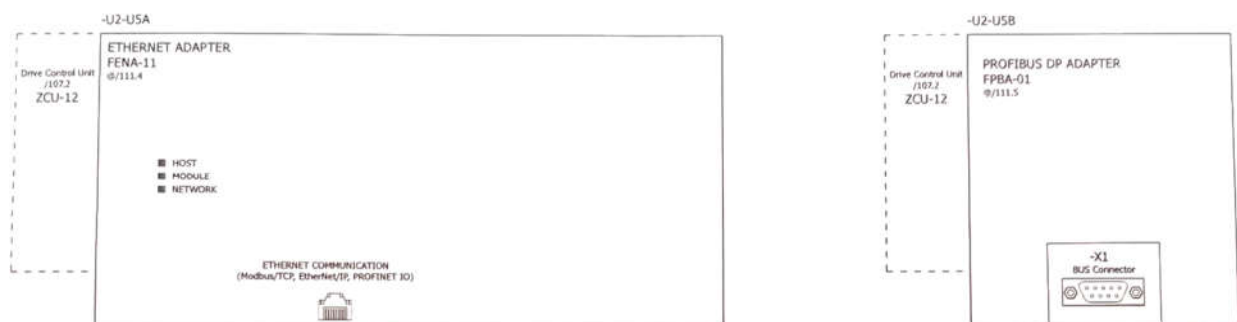
Sl. 4.5. Shema Profibus i Ethernet adaptera
