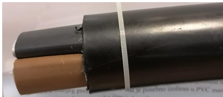
Slika 7.9: Kabel – NAYY-J 4 \times 150 \text{mm}^2
