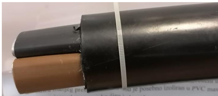
Slika 7.9: Kabel – NAYY-J 4 \times 150 \text{mm}^2
