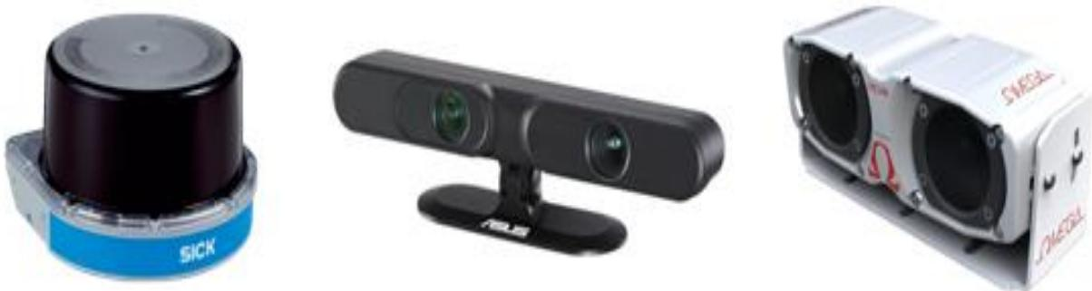
Slika 2.1 LIDAR (Sick), RGB-D kamera (Asus Xtion Pro) i stereo kamera (Omega).
