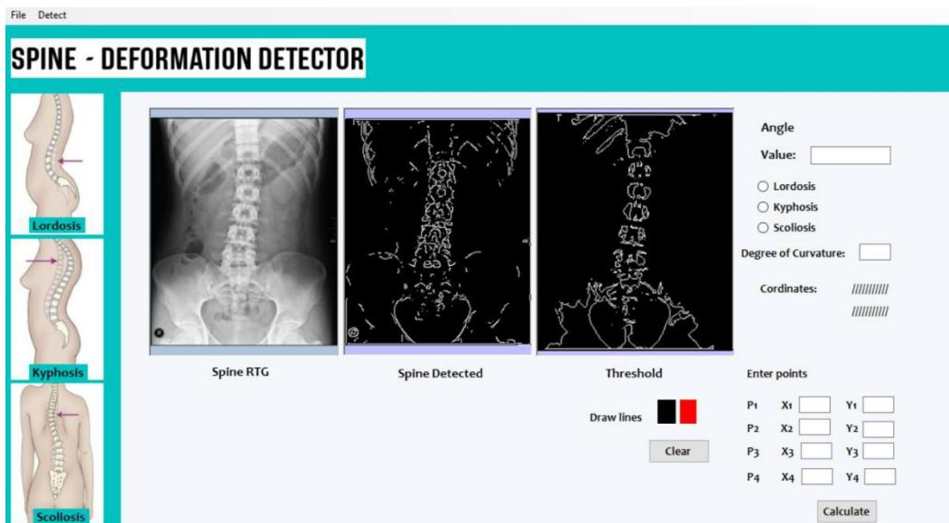
Slika 4.7 Canny metoda u usporedbi s Threshold metodom
