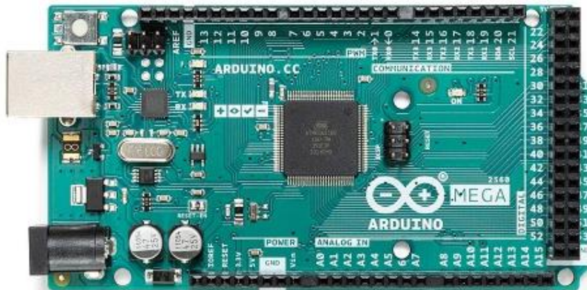
Sl. 3.2. Arduino Mega platforma [7]
