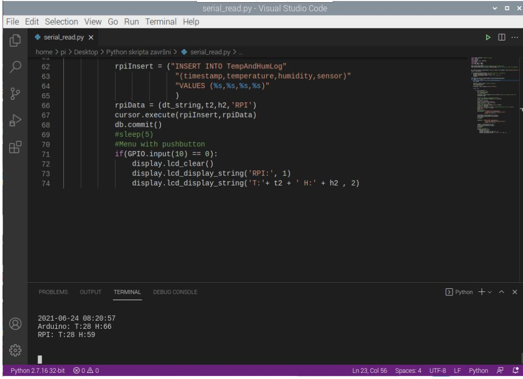
The screenshot shows the Visual Studio Code interface with the file `serial_read.py` open. The code reads data from the serial port, inserts it into a MySQL database, and updates an LCD screen. The terminal window shows the current date and time, and the output window shows the data being inserted into the database.
