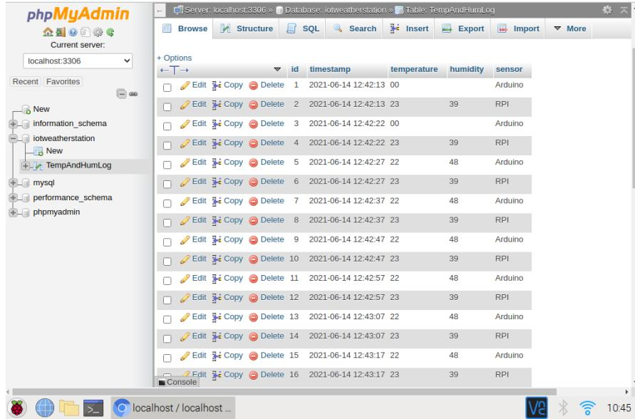
The screenshot shows the phpMyAdmin interface connected to a MySQL database named 'iotweatherstation'. The 'TempAndHumLog' table is selected. The table has columns: id, timestamp, temperature, humidity, and sensor. There are 16 rows of data, each representing a measurement from either an Arduino or a RPI. The data is as follows:
