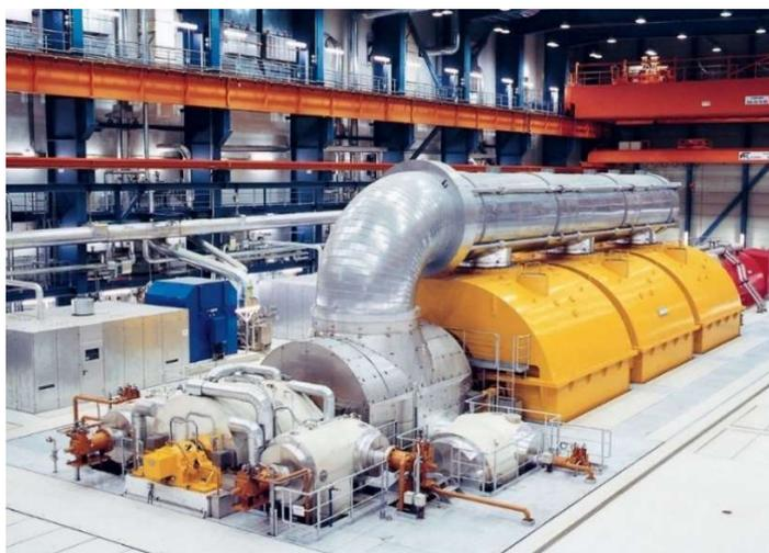
Slika 3.3 Siemens turbogenerator snage 500 MW, pokretan parnom turbinom [8]
