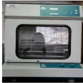
Sl. 2.1. Tresilica-inkubator marke Edmund Bühler TH15.
