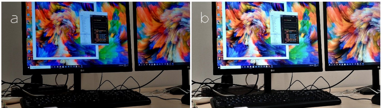
Figure 2: Brightness equalization of the darker image from figure 1 with gain equal to 1.413963 and bias equal to 13.771867 (a – Original image, b – Brightness equalized image using basic linear transformation)
