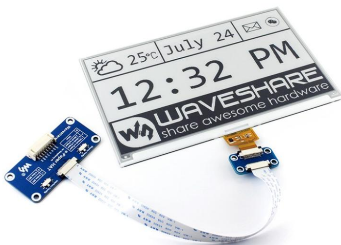
Slika 3.6. Waveshare 7.5inch e-Paper HAT [13]
