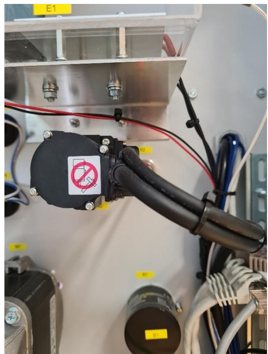
Sl. 2.19 Servomotor HG-KN13J
