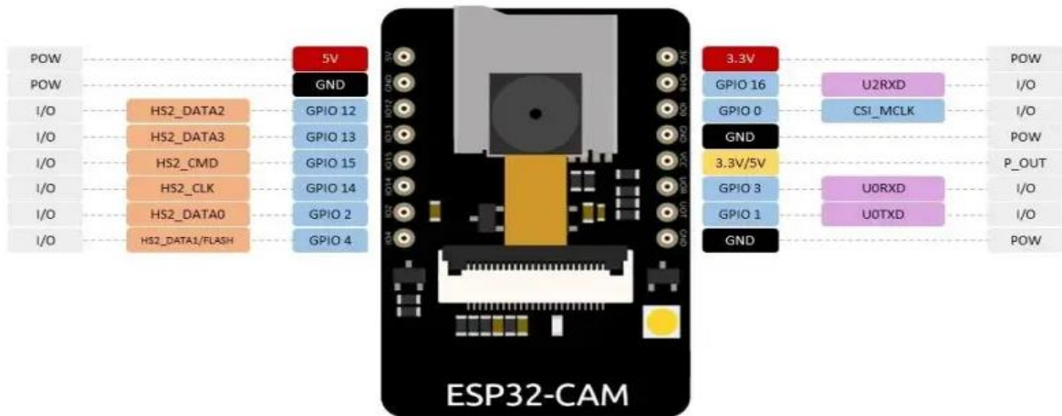
Sl. 3.2. Raspored pinova ESP32-CAM [11].
