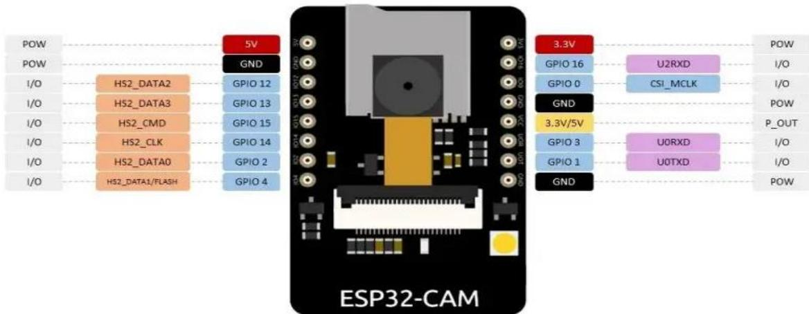
Sl. 3.2. Raspored pinova ESP32-CAM [11].
