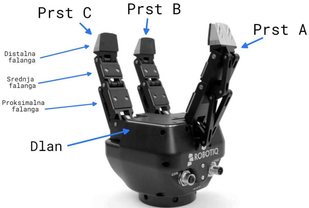
Sl. 4.3: Robotiq 3-Finger robotska šaka [35]
