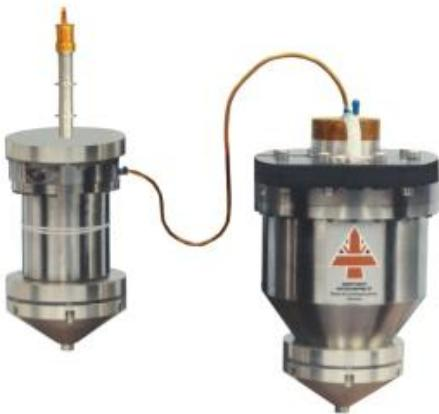
Slika 7.2. British Aerospace 50-80 K cryocooler
