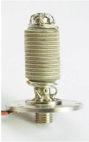
Slika 5.2. Grafički prikaz Joule-Thomsonovog *cryocoolera* (*Fast Cool Down Joule-Thomson Miniature Cyogenic Cooler*).
