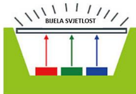
Slika 4.4. Crveni LED + plavi LED + zeleni LED [32]
