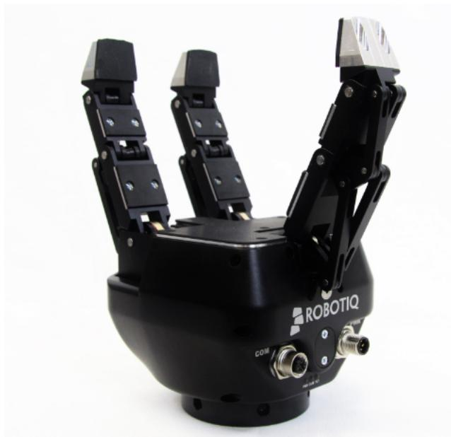
Slika 4.5: Robotiq 3-Finger Gripper. [14]
