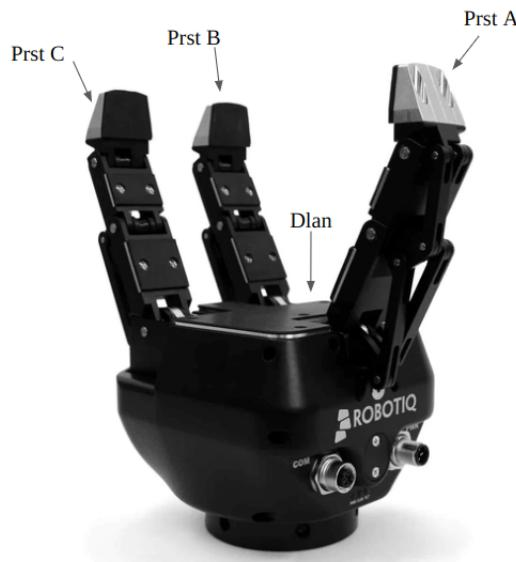
Slika 4.6: Robotska hvataljka Robotiq 3-Finger Adaptive Robot Gripper [12]
