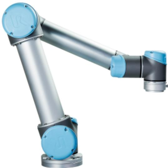
Slika 4.5: *Robotski manipulator UR5 [9]*
