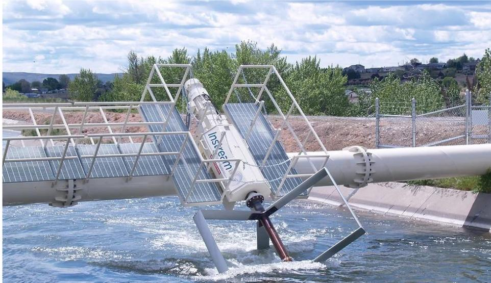
*Slika 3.27. Instream Energy Systems H-Darrieusova turbina [36]*
