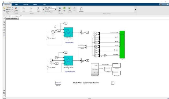
**Slika 3.2.** Simulacijski model jednofaznog asinkronog motora unutar Matlaba (H. Ouquelle and Louis-A.Dessaint (Ecole de technologie superieure, Montreal))<sup>[7]</sup>
