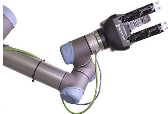
Slika 5.3 Universal Robots Robotiq 3-Finger hvataljka
