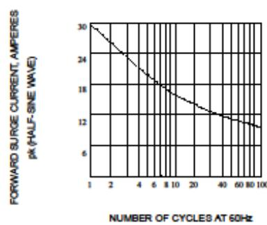
Fig. 3-MAXIMUM NON-REPETITIVE FORWARD SURGE CURRENT
