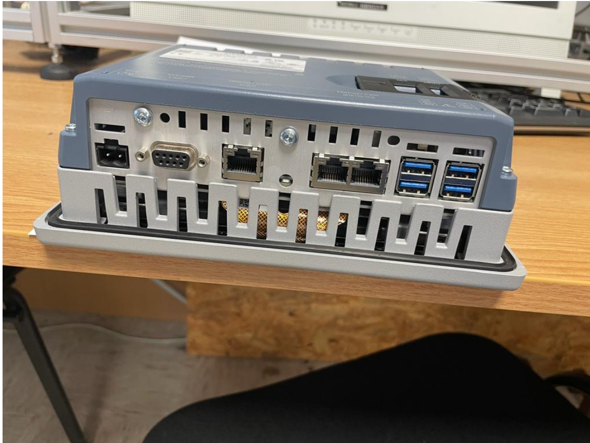
Sl. 5.2. Stražnja strana Siemens Simatic MTP700 unified comfort panela
