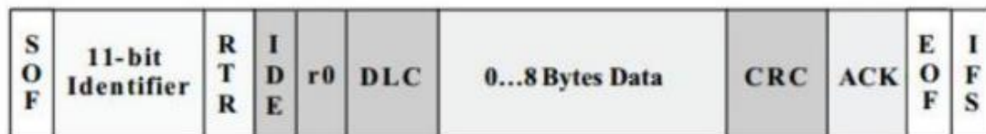
Figure 7.1: Standard CAN Frame Format
