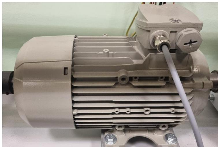
Slika 3.1 Siemens 1FK7 sinkroni motor s permanentnim magnetima
