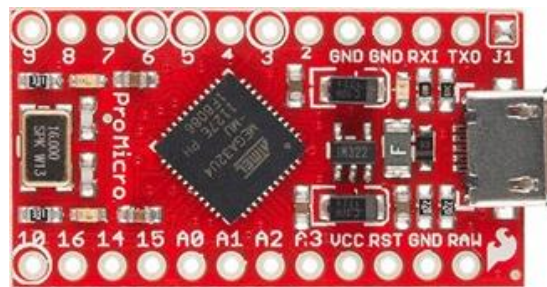
Sl. 3.3. Arduino ProMicro 5V/16MHz
