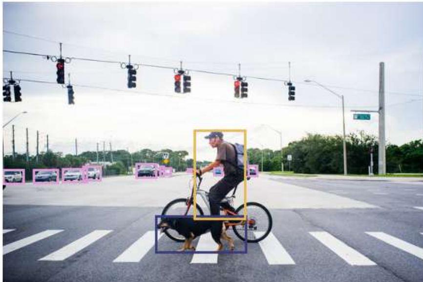
Figure 2.1: An example of object detection in an autonomous driving scenario (Lin et al., 2014). The vehicle detects and localizes a pedestrian, a dog, and several cars.
