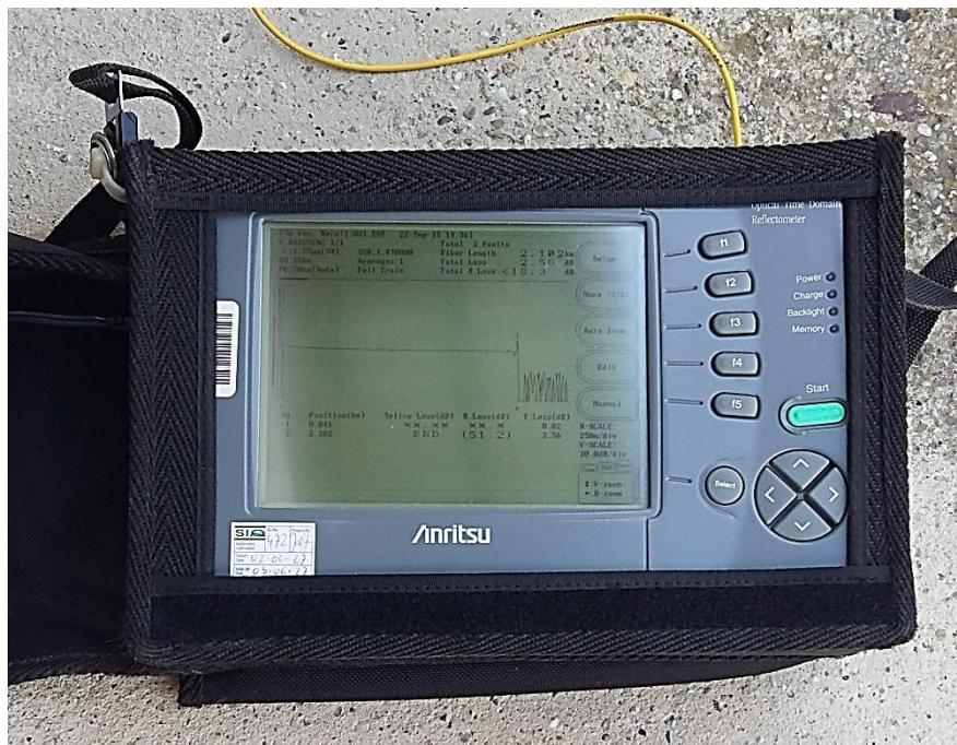
Slika 4.3 Mjerni instrument OTDR Anritsu MW9070B
