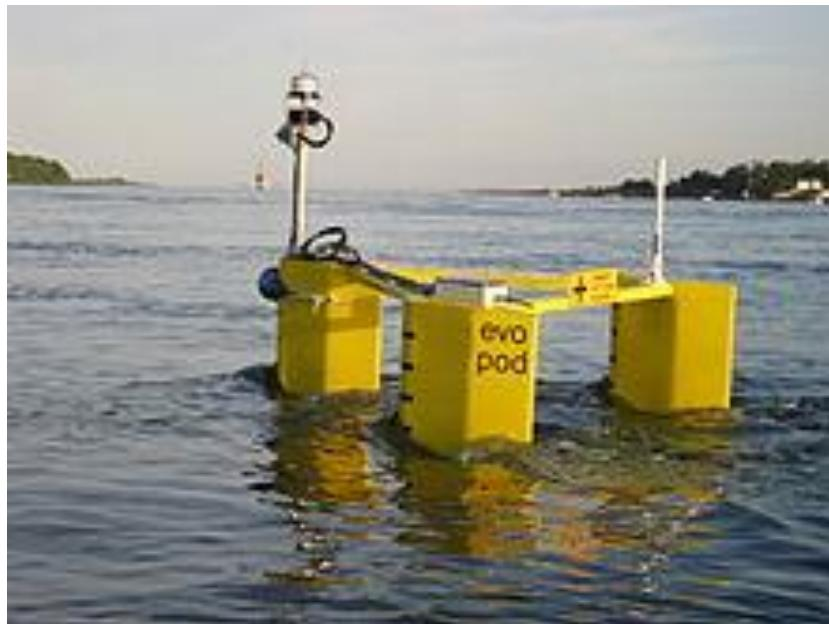
**Slika 6.3.** Prototip turbine Evopod
