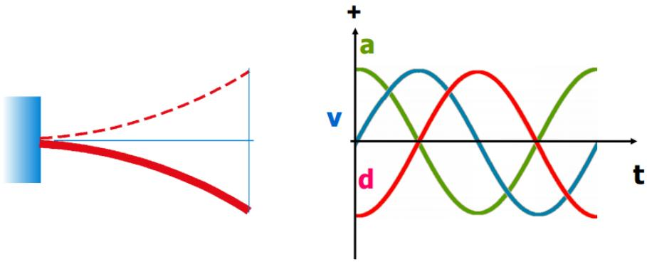
$$\begin{aligned} \textcolor{red}{d} &= \text{mm} \\ \textcolor{blue}{v} &= \text{mm/s} \\ \textcolor{green}{a} &= \text{mm/s}^2 \end{aligned}$$
