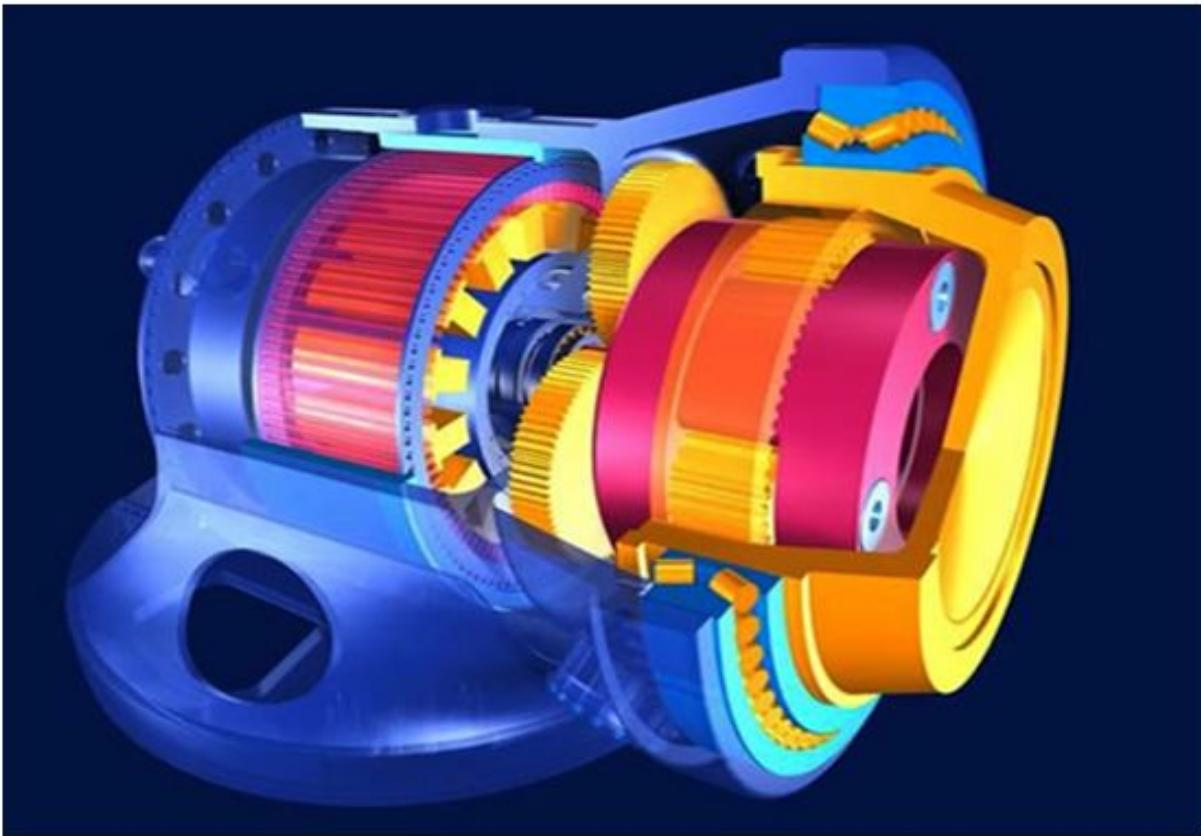
Sl. 4.6 Presjek generatora s permanentnim magnetima, [12]
